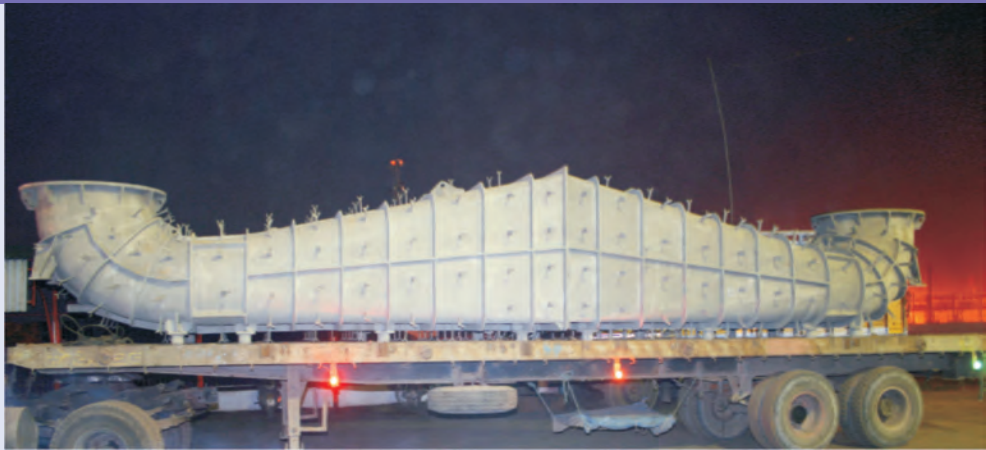
Draft Tube for 13 MW pump (Wt. 5.35 Tonnes)
